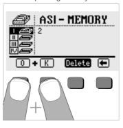
A security query is displayed if the Delete key is activated from the ASI-MEMORY menu: The 0 and K keys must be activated simultaneously in order to acknowledge deletion of the contents of the memory, or the selected memory address.
