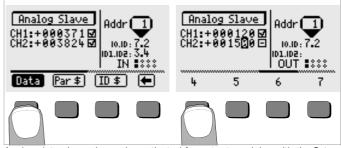
Analog data channels can be activated for output modules with the Data key, and transmitted to the slave after acknowledgement. Numerals which do not appear initially can be displayed by pressing the
