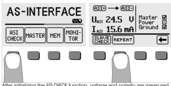
After initializing the ASI CHECK function, voltage and polarity are measured. If no external AS-i voltage is detected, power is supplied by the METRAtest 36ASi, which allows for measurement of current consumption for the AS-i slaves.
