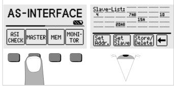
After initializing the MASTER function, addresses are listed for all of the slaves at the AS-i bus.
