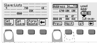
After the Set Addr. function has been initialized, new addresses can be assigned to individual slaves. After selecting the slave address to be changed with the Prev. or the Next key and acknowledging with the Lakey, a list of all currently available slave addresses is displayed.
