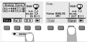
After selecting an analog slave, the slave's analog channels are displayed at the left, and abbreviated slave data appear at the right. The display can be switched to the diagnosis string (if available), as well as to the name entry menu and back to the main menu with the and keys at the toggle switch. After activating the Name key, the instrument is switched to the alphanumeric entry mode as described in chapter 7.3.
