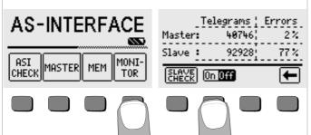
The system tester functions as a passive bus user in this operating mode. The instrument detects bus system errors separately for slaves, and for the master. The error quota is calculated as a percentage of the total number of telegrams (from the master and the slaves).
