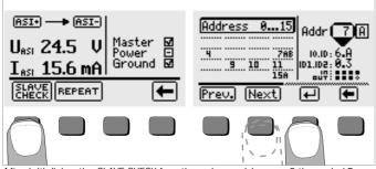
After initializing the SLAVE CHECK function, slave addresses 0 through 15 are displayed along with the abbreviated data from the slave with the lowest address. The display can be switched back and forth between address ranges 0 through 15 and 16 through 31 with the ← or the → key at the toggle switch. The desired slave address from either of the address ranges is selected with the Prev. or Next key, and is acknowledged with the ↓ key.
