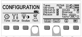
The self-test is started from the main menu with the Test key. The test has a duration of several minutes. The following information is displayed in the two headers:
