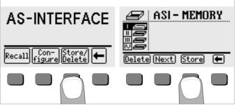
After activating the Store/Delete key once, the desired memory address (I, II, III or IV) must first be selected with the Next key, to which the slave addresses which are now in RAM are to be stored. After activating the Store key a second time, a list of all stored slave addresses is generated. If the Store key is activated again, a menu appears for the entry of a new system name, or a new AS-i bus name for the previously selected memory address.
