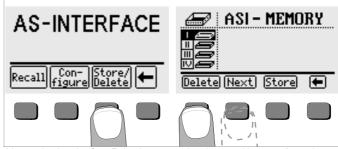
After activating the Store/Delete key, a previously stored bus configuration or the corresponding memory address can be selected with the Next key.
