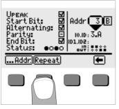
If only one slave has been connected to the bus, the above described selection menu does not appear. The slave's telegram data are displayed, which allows for conclusions regarding possible data transmission errors.
