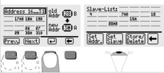
The display can be switched back and forth between addresses ranges 0 through 15 and 16 through 31 with the  $\leftarrow$  and the  $\Rightarrow$  keys at the toggle switch.
