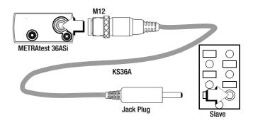
The necessary connections have now been established, and addressing can begin with the METRAtest 36ASi addressing and test instrument.
