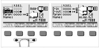
The hourglass and the arrow indicate transmission to the slave and updating of the **D-in** inputs. Key operations are disabled during transmission of parameters and data. This is indicated by means of dashed softkeys.
