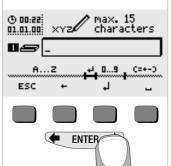
Display the desired alphanumeric character by pressing the ← or the → key at the toggle switch and select it with the corresponding softkey. Control characters are entered in the same way and have the following meanings: ←: delete in reverse, ¬!: new (second) line, otherwise identical with the ENTER key, ESC: exit entry mode without saving data. Each time a character is selected, the cursor moves one place to the right. Previously entered characters can be deleted in reverse by
