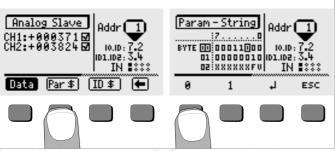
Beyond this, the parameter string (Par \$) can be queried or edited, and the ID string (ID \$) can be read out. After the parameter string has been edited, the new values are transmitted directly to the slave. Switching is possible between bytes 00 through 02, 03 through 05, 06 through 08 and 09 through 11 with the Prev. or Next key, or with the  $\longleftarrow$  or  $\Longrightarrow$  key at the togale switch.
