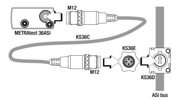
The necessary connections have now been established, and testing can begin with the METRAtest 36ASi addressing and test instrument.
